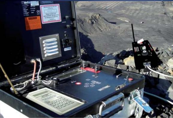
After successful field evaluations in large open-pit operations, Davey Bickford announces the introduction of the Daveytronic® **Wireless Blasting System**. The new system allows technicians to remotely detonate single or multiple shots from a distance of up to 1.5 mile (2.4 km) away from the pattern, significantly improving **safety** during the blast and exceeding minimum distance requirements.
